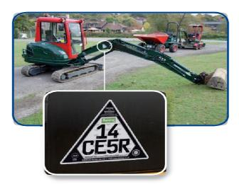
If the mini-excavator is left overnight, remove it from the trailer. Slew the cab 90° and extend the boom arm. Use immobilisers and / or hydraulic locks. This makes the machine impossible to remove or lift away. Note the presence of an approved registration scheme, (e.g. The CESAR Scheme) and corporate identity. Criminals dislike stealing this type of equipment due to the expense of changing the unique branding.
