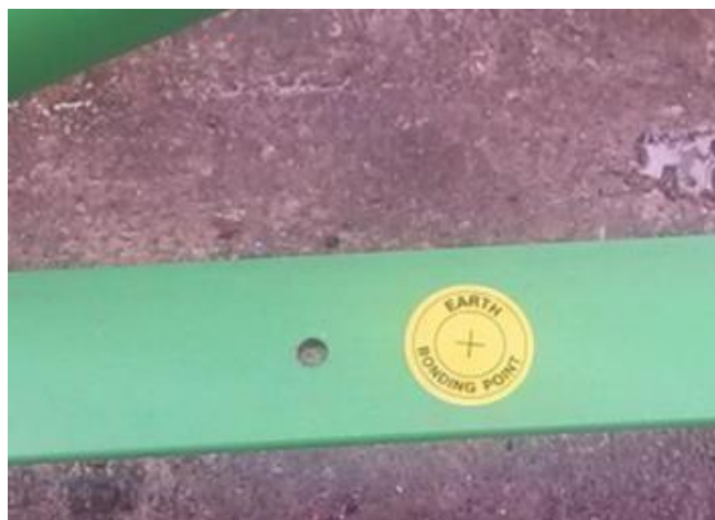
Figure 1: Earthing point marked by manufacturer.
