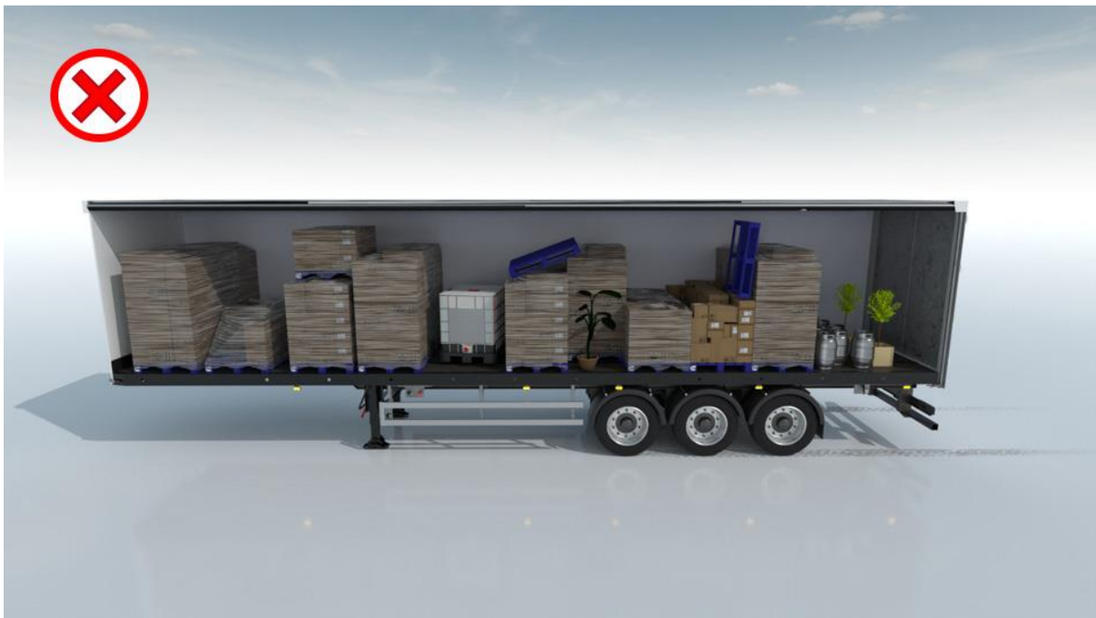
An example of a load that does not positively fit the trailer - there are gaps in the load and different types of goods which will move during transit.
