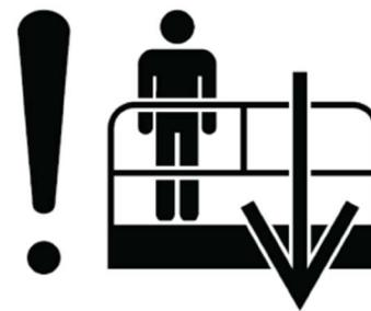
A decal may be positioned directly above or in the vicinity to identify the location of the emergency/auxiliary lowering controls
