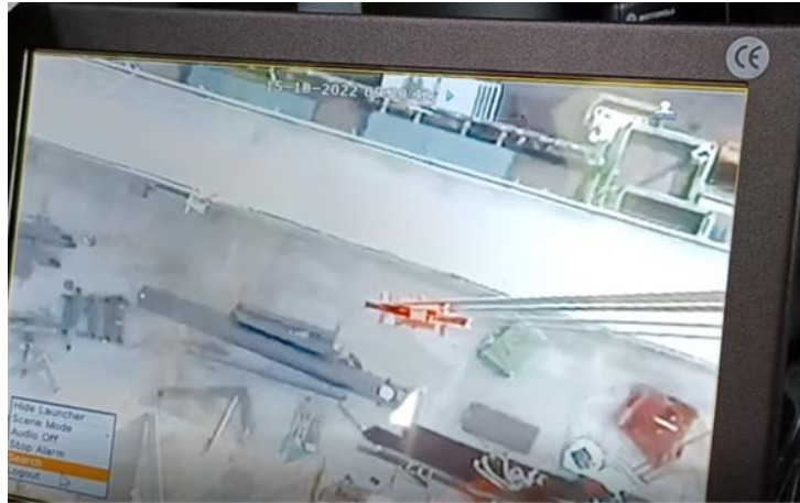
Figure 2: View from jib mounted camera.
