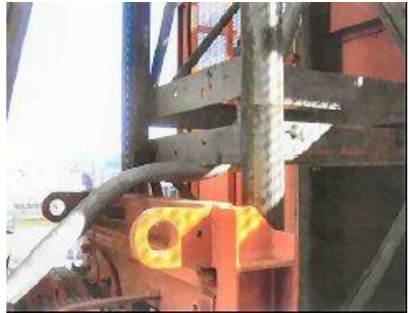
Close-up of damage caused by unsecured tube.
