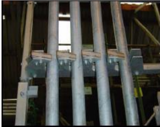
Examples of Scaffold Tubes Held Securely Top and Bottom
