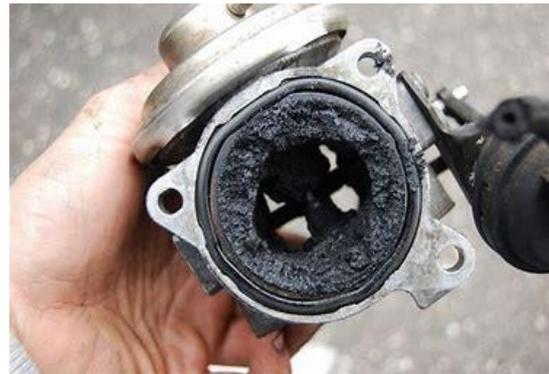
**Blocked Exhaust Gas Recirculation Valve**
