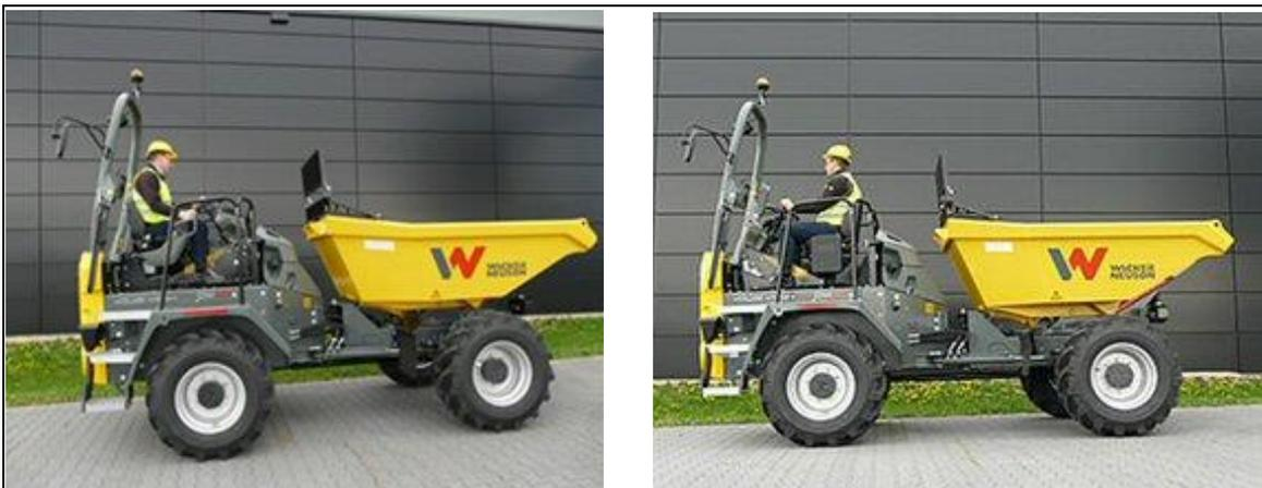
**Figure 18 – Example of a Reversible Seat Dumper**
