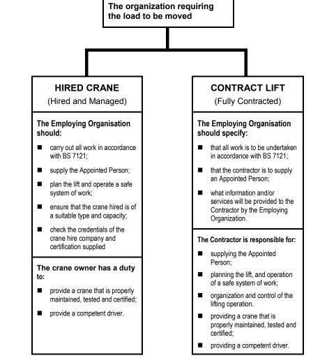
Where a tower crane is being hired in by a contractor, the erection and dismantling of the crane will be carried out by the tower crane supplier who has overall responsibility for the operation. Once the tower crane has been erected, thoroughly examined and handed over to the Contractor (Hirer) then all lifting operations using that crane are the sole responsibility of the Hirer as summarised in the left hand column (Hired Crane) of the diagram above.
