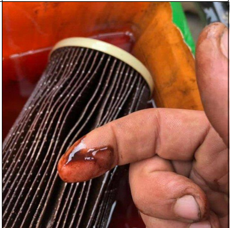
Blocked Fuel Filter
