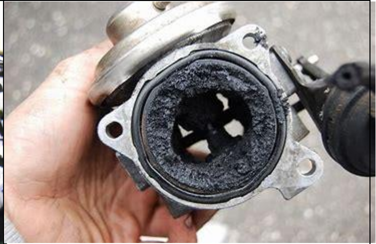
Blocked Exhaust Gas Recirculation Valve
