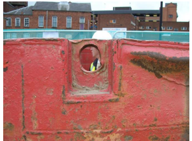
Figure 4 - Stretching of the hole edges
