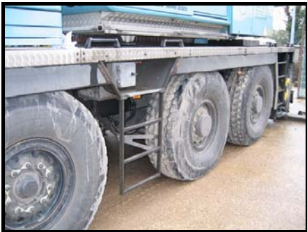
Fig. 1 - Additional Access Ladders
