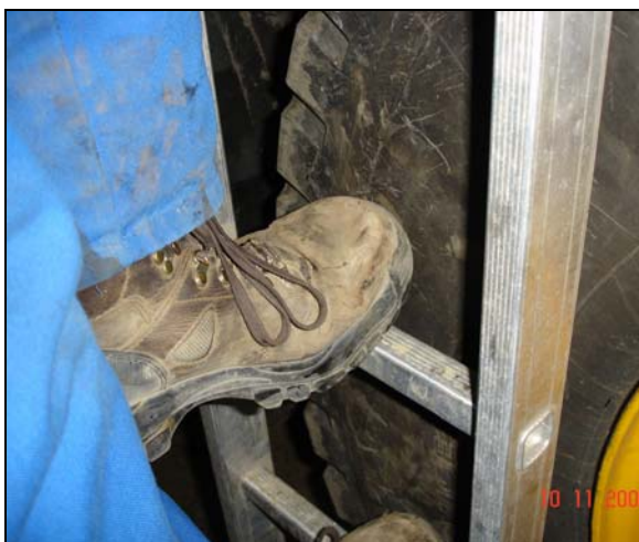
Fig. 2 - Insufficient Foot Penetration
