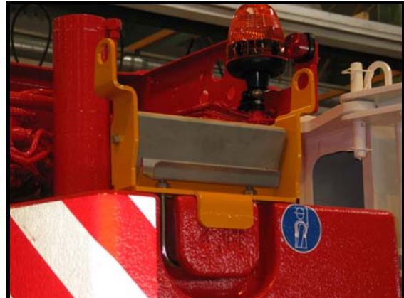
Automatic Ladder Latch with Anchor Point
