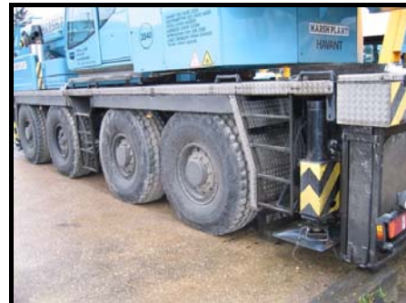
Fig. 2 - Additional Access Ladders
