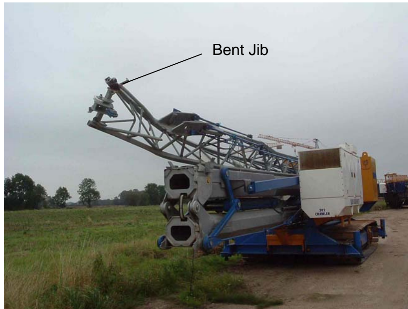
An operator who had not received training on the manufacturer's dismantling procedure attempted to dismantle a SETC in high winds. During the dismantling process the jib was damaged.
